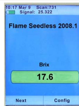
An example PHAZIR screen showing the result of a Brix measurement on a grape.
